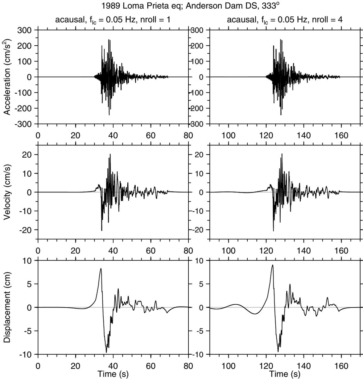
Fig. 1. Comparison of acceleration, velocity, and displacement for an acausal 0.05 Hz low-cut filter with  $nroll = 1$  and  $nroll = 4$ . The time axis includes the pads (30 sec and 120 sec of pre-event pads for the  $nroll = 1$  and  $nroll = 4$  cases, respectively). Note the ringing in the displacement record for  $nroll = 4$ .
