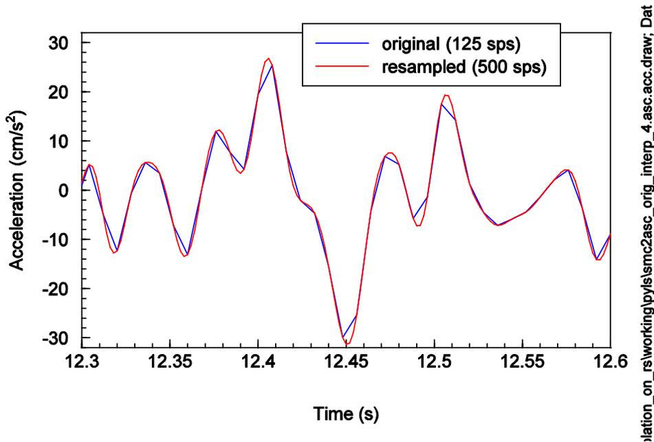
Figure 8. A small portion of the original and resampled acceleration in the vicinity of the absolute peak acceleration.
