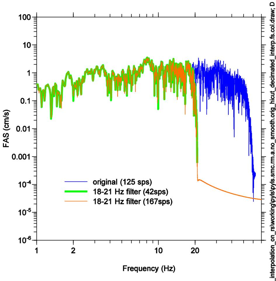
Figure 10. FAS of the original PYLS record and the simulated anti-alias filtered and low sample rate recorded record (and with the resampled version of that simulated record).
