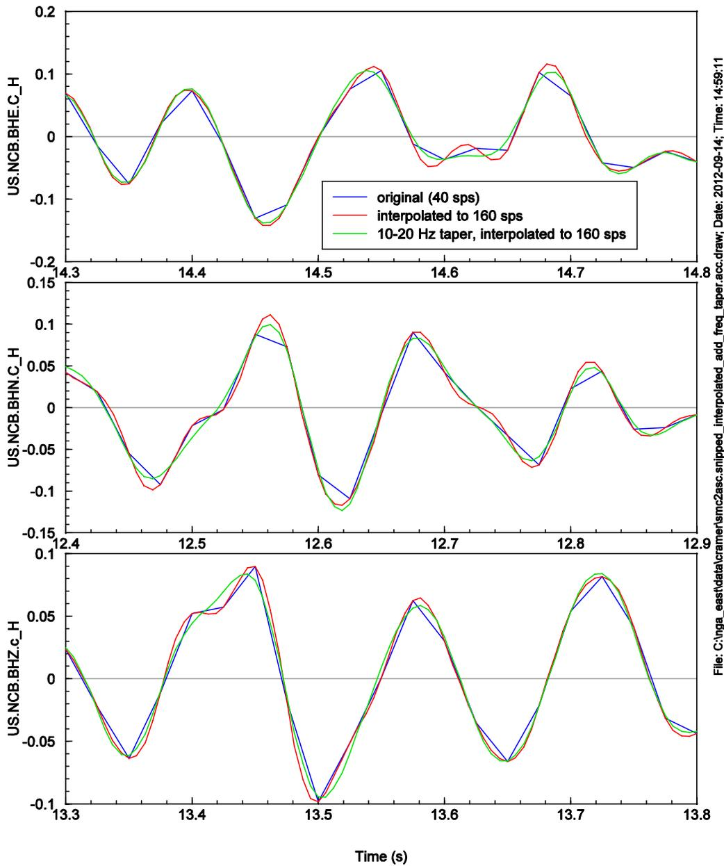
Figure 5. Original and resampled time series (the FAS taper from 10 to 20 s changes the time series, even without resampling, so that it no longer necessarily coincides with the original time series at the sample times).
