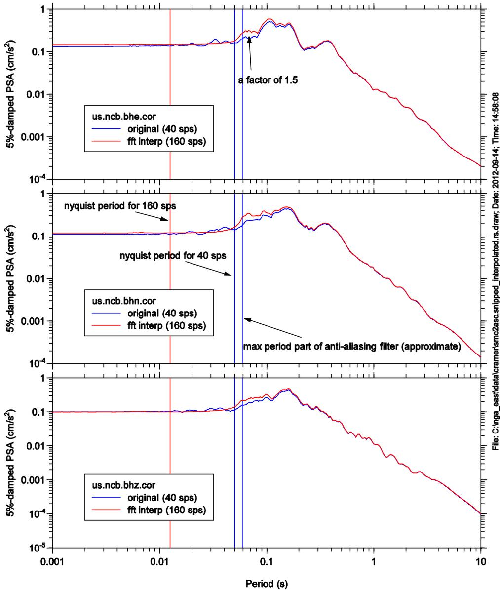
Figure 3. 5%-damped PSA for the original and resampled time series. For reference, the vertical lines show the periods corresponding to the Nyquist frequencies of the original and resampled time series. Also shown is the period corresponding to the frequency at which I estimate the anti-aliasing filter started (about 17 Hz).
