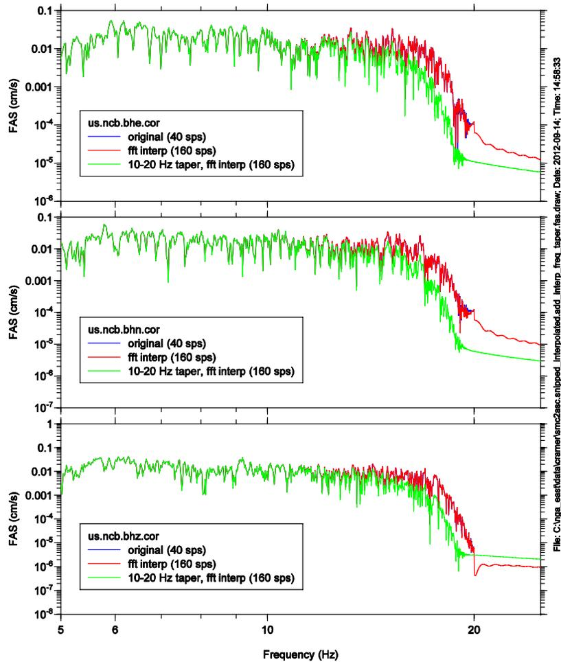
Figure 4. FAS of original and resampled time series, without and with an additional taper from 10 to 20 Hz.
