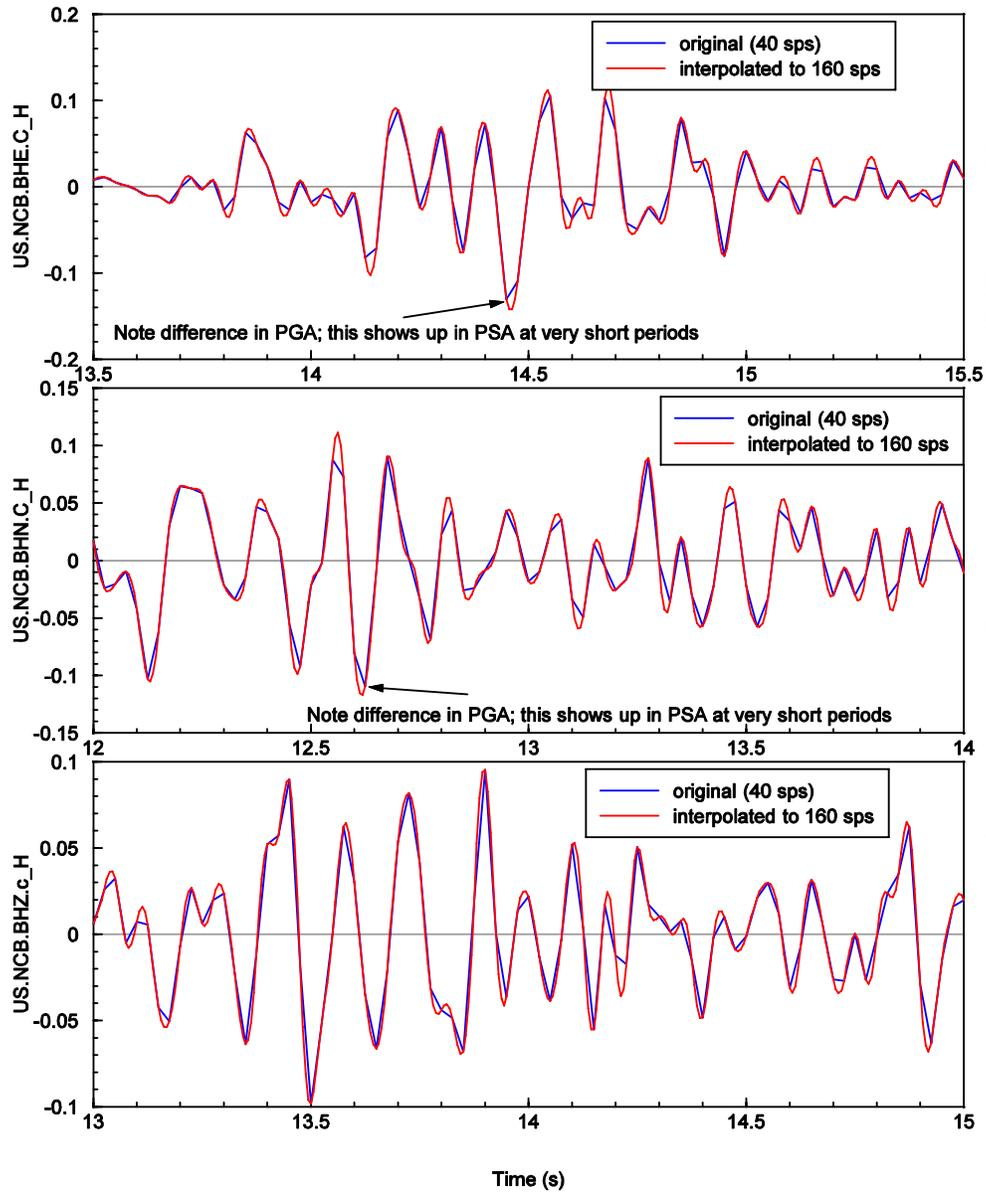
Figure 2. The portions of the records containing the absolute peak motions, comparing the straight line and sampling theorem interpolations.
