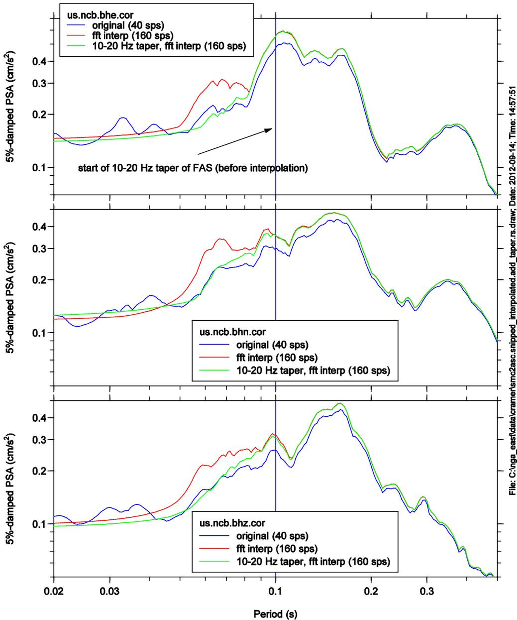
Figure 6. PSA for the three time series. The vertical blue line is corresponds to the lowest frequency of the 10 to 20 Hz taper applied to the FAS of the original records.
