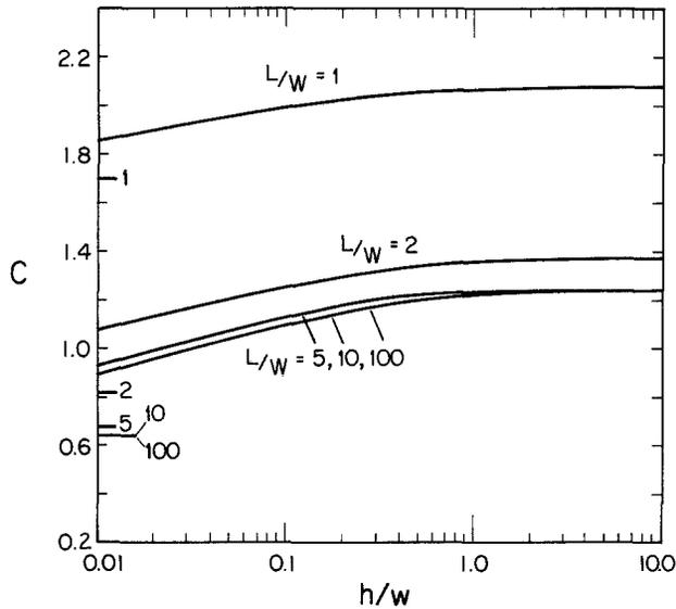
FIG. 1. Shape factors for a vertical strike-slip fault as a function of normalized depth of burial for various  $L/W$  ratios, assuming a constant stress drop over the fault surface. The  $h/W = 0$  values are indicated by tick marks.
