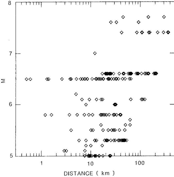
FIG. 8. Distribution in magnitude and distance of the peak horizontal acceleration data used by Joyner and Boore (1981). Each point represents one recording.
