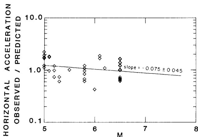
FIG. 15. Residuals of peak horizontal acceleration with respect to the predictions of Joyner and Boore (1981) for recordings within 10 km of the fault.
