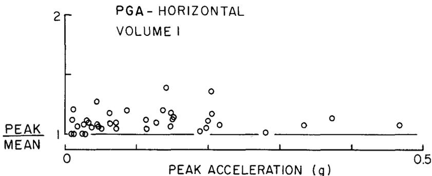
FIG. 1. Ratio of larger peak ground acceleration (PGA) on either horizontal component to mean of the two peaks. Points correspond to those recordings in the data set of Joyner and Boore (1981, Table 2) that are contained in volume 1 of the series "Strong Motion Earthquake Accelerograms," published under the direction of D. E. Hudson by the Earthquake Engineering Research Laboratory of the California Institute of Technology.
