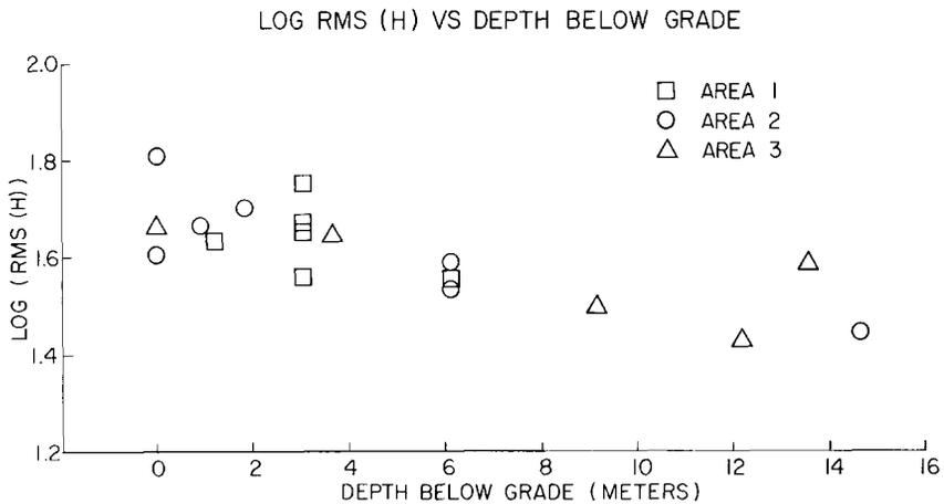
FIG. 6. The dependence rms acceleration on embedment depth of instrument for data recorded in three small areas in Los Angeles during the 1971 San Fernando earthquake (from McCann and Boore, 1983).
