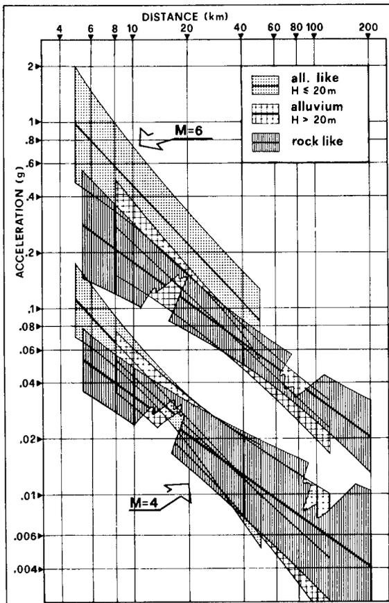
FIG. 7. Attenuation relations for data from Friuli, Italy, showing the tendency for motions on shallow soil sites to be larger than on either rock or deep soil sites (from Chiaruttini and Siro, 1981). Cutaways expose patterns on obscured fields.
