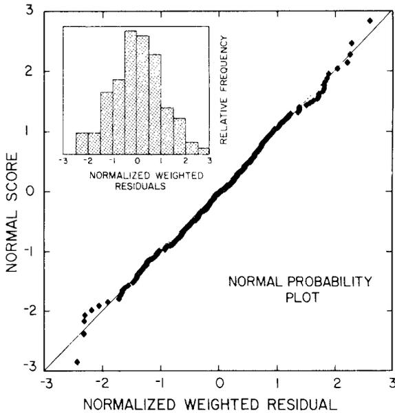
FIG. 9. Normal probability plot of residuals of the logarithms of peak acceleration around the prediction equation of Campbell (1981b); this evidence for a log-normal distribution of peak ground acceleration is confirmed by a Kolmogorov-Smirnov test at the 90 per cent confidence limit (after Campbell, 1981b).
