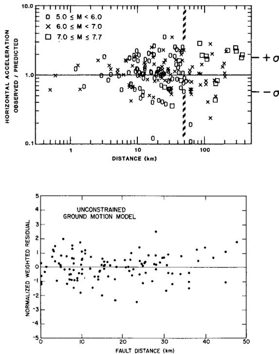
FIG. 14. Residuals of data about predictions: (*top*) from Joyner and Boore (1981); (*bottom*) from Campbell (1981b). Heavy dashed line in *top graph* marks 50-km distance from fault for ease in comparing with *bottom* residuals, which extend out to 50 km only. Campbell's residuals have been normalized by the standard deviation (0.16 log units).
