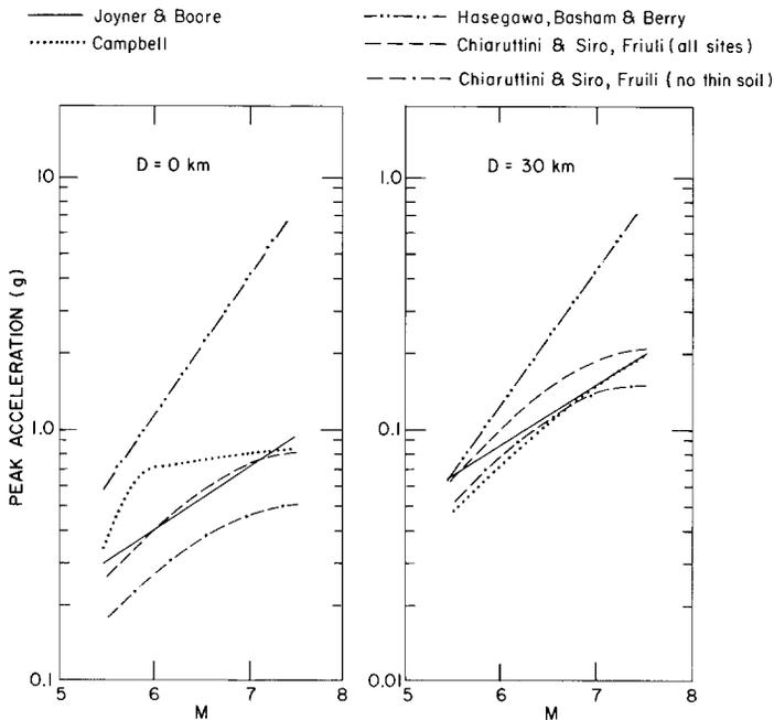
FIG. 11. Comparison of peak horizontal acceleration predictions for various papers in the December 1981 issue of the *Bulletin of the Seismological Society of America*. For the Campbell prediction, the *top edge* of the fault was assumed to be at 2.5-km depth for  $M = 5.5$  and to break the surface for  $M = 6.0$ . See the text for other assumptions made (see Swanger *et al.*, 1980 for a similar figure comparing earlier predictions).
