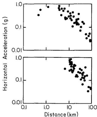
FIG. 4. Horizontal acceleration data from the 1979 Imperial Valley earthquake plotted against shortest distance to fault (*top*) and distance to a point along the Imperial fault about 16 km northwest of the epicenter (*bottom*, both from Shakal and Bernreuter, 1981).
