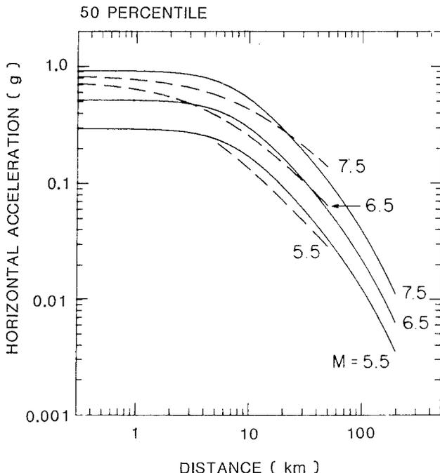
FIG. 13. Comparison of attenuation curves for peak horizontal acceleration by Campbell (1981b) (dashed lines) with the 50 percentile curves by Joyner and Boore (1981) (solid lines). Campbell's curves are raised by 13 per cent to compensate for the fact that he took horizontal acceleration as the mean of the peaks on the two horizontal components. Magnitudes at *right ends* of curves.
