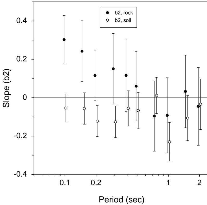
Figure 2. Slopes of the regression of residuals to the Boore et al. (1994) relationship for rock and soil sites against predicted response at rock sites, plotted against period. The bars show the standard errors of the slopes. (Both the rock and soil symbols have been offset horizontally for clarity.)
