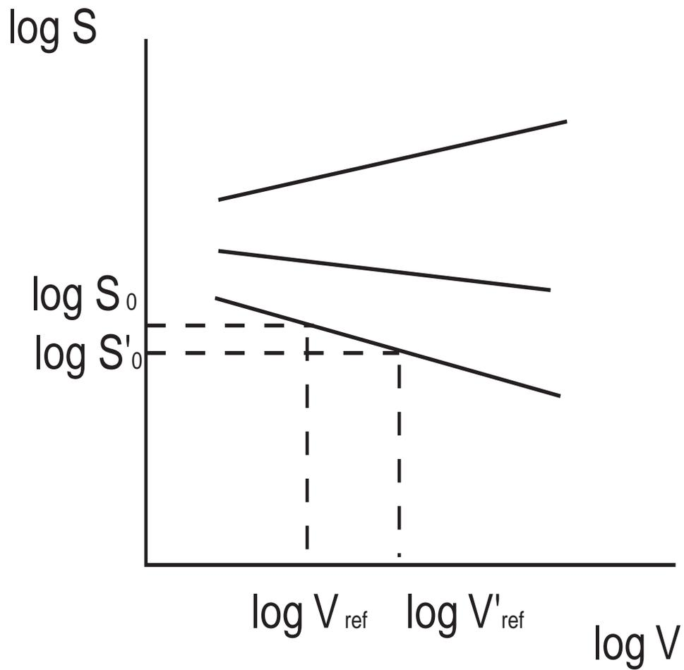
Figure 1. Changing the reference velocity from  $V_{ref}$  to  $V'_{ref}$ . The response value  $S'_0$  at  $V'_{ref}$  corresponds to the value  $S_0$  at  $V_{ref}$ . The solid lines show the relationships between  $\log S$  and  $\log V$  for given values of  $S_0$ .
