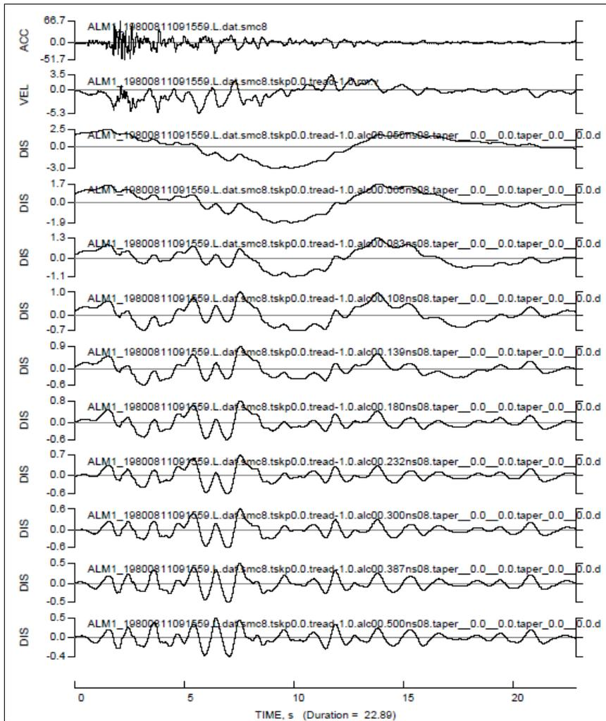
Figure 3. Displacement time histories for a specific accelerogram corrected by various  $f_c$  values (logarithmically equally spaced) from 0.05 to 0.50 Hz. The same procedure is repeatedly applied for 0.1 to 1.0 and 0.5 to 5.0 Hz for each component as well.
