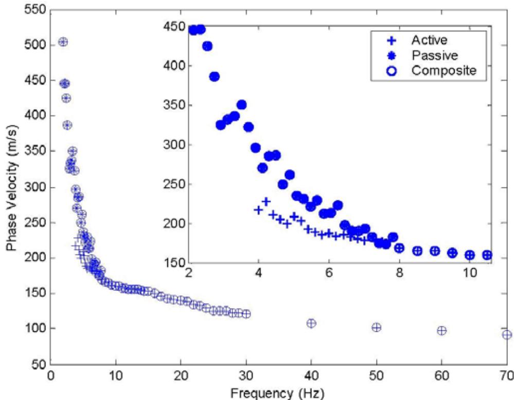
Figure 4. Dispersion curves from active and passive sources (from Yoon and Rix, 2005). The inset shows detail for periods less than about 10 Hz.
