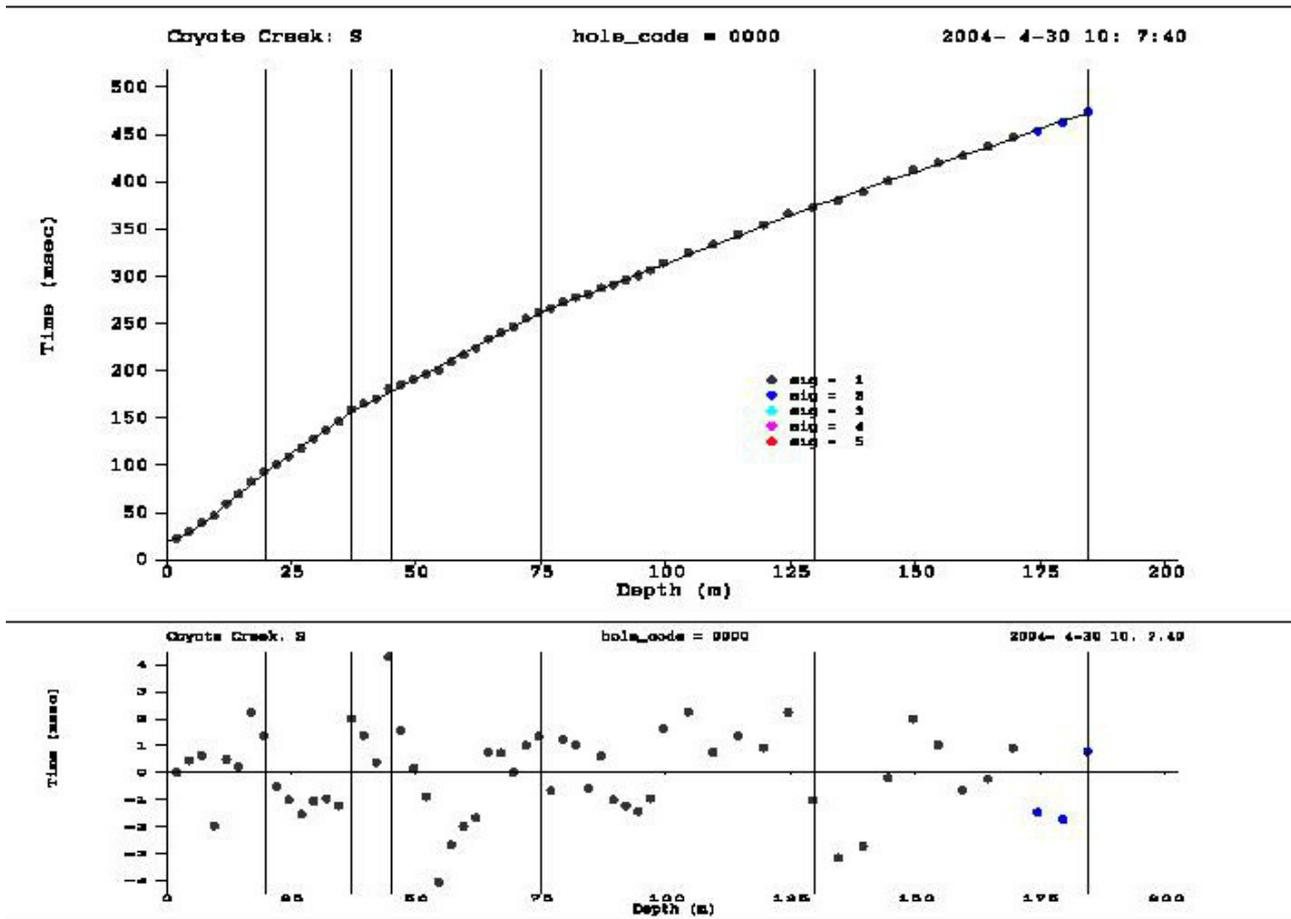
Figure 3. Fit to S-wave travel times for record section from CCOC. The depth is vertical depth in the borehole, but the travel times are from a surface source offset a few meters horizontally from the borehole---for this reason, the travel times are not zero for zero depth.
