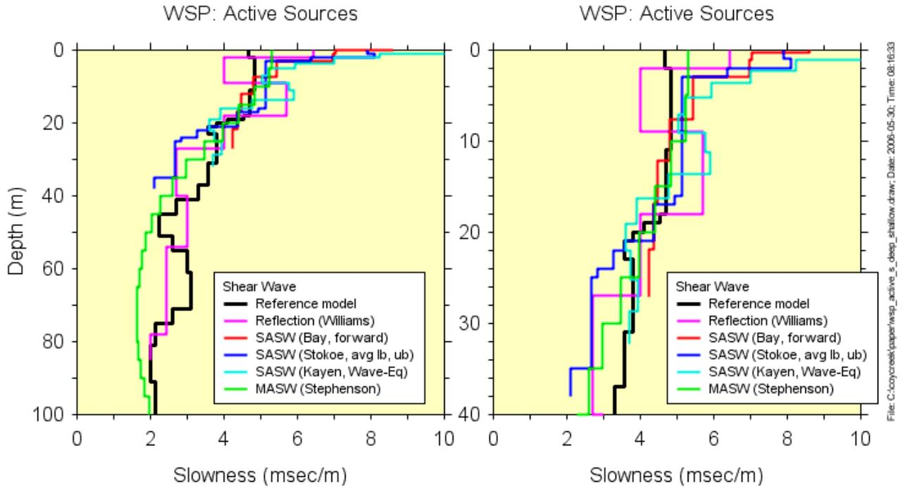
Figure 9. Comparison of reference model and models from active source measurements at WSP. An expanded depth scale is used in the right-hand graph to show better the details at shallow depths.
