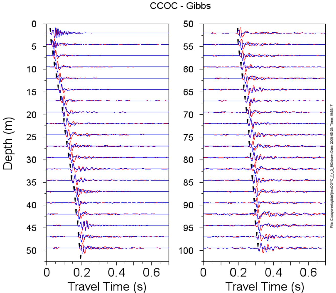
Figure 2. Record section at CCOC for surface source—downhole receiver method. The red and blue traces correspond to opposite directions of impact of the shear-wave source (although some polarity errors have resulted in similar polarities at some depths in the plot). The picked travel times are indicated by the small wedges (after Gibbs, personal communication; see also Boore, 2003a).
