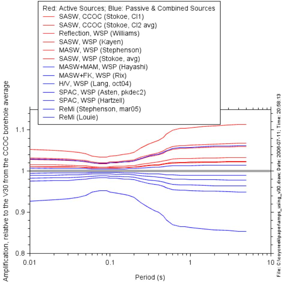
Figure 14. Amplifications based on equation used in recent empirical ground-motion estimation models. No amplifications are given for Bay et al. because their preferred models did not reach 30 m. I have used different colors for models from active and for passive (including combined) sources. The differences in amplifications are very small.
