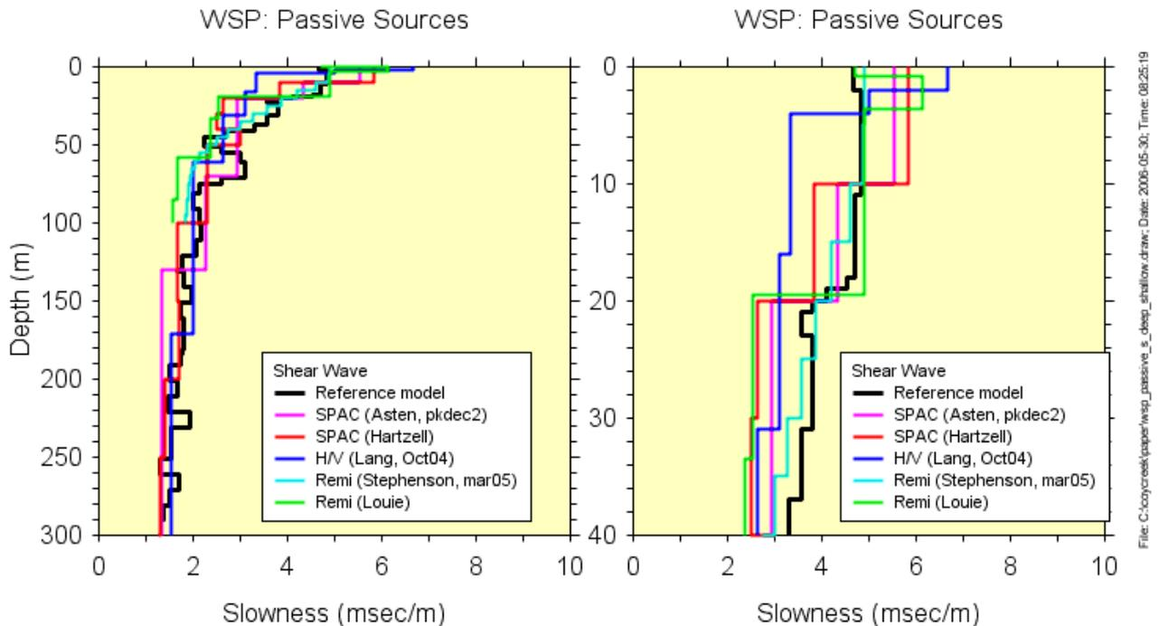
Figure 10. Comparison of reference model and models from passive source measurements at WSP. An expanded depth scale is used in the right-hand graph to show better the details at shallow depths.
