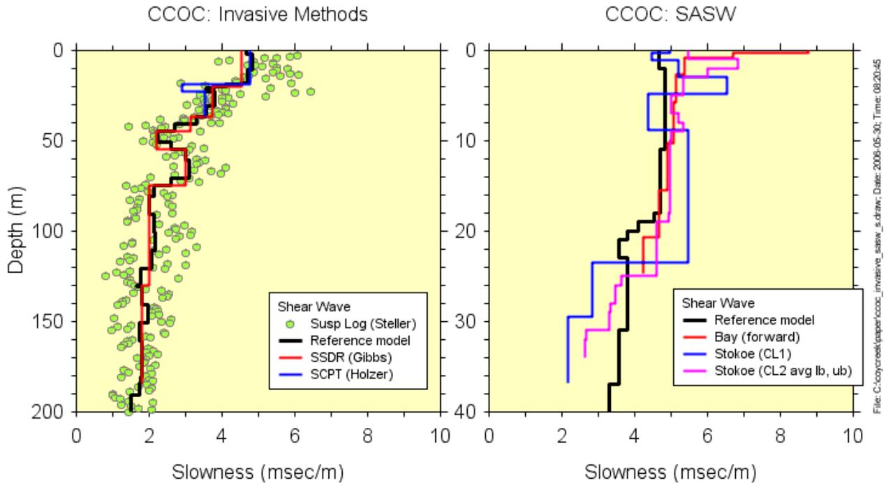
Figure 8. Comparison of reference model with models from invasive and noninvasive measurements at CCOC.
