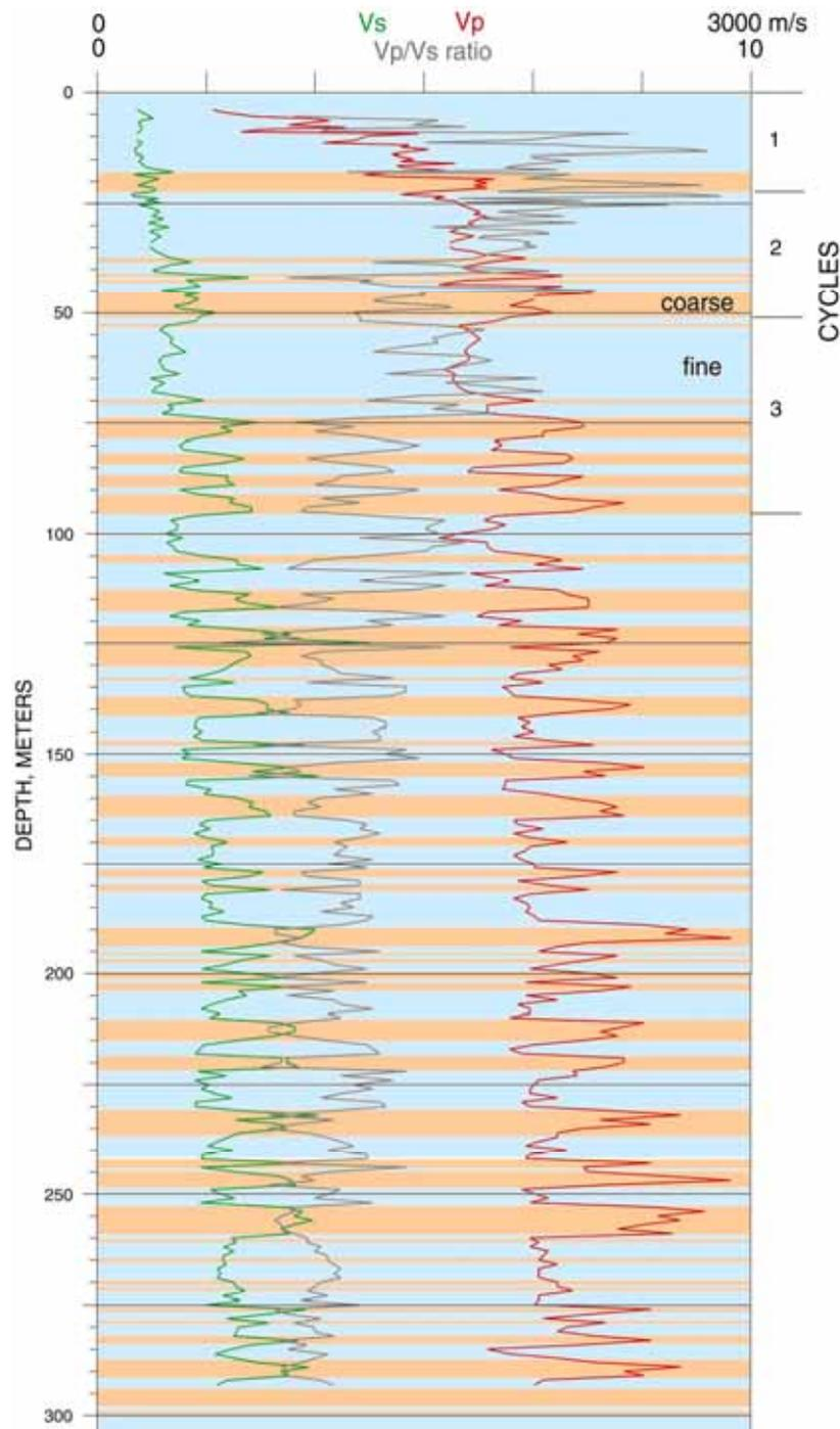
Figure 6. Seismic velocities from suspension PS log and simplified lithology, from Wentworth and Tinsley (2005). The blue and orange colors represent fine- and coarse-grained sediments, respectively.
