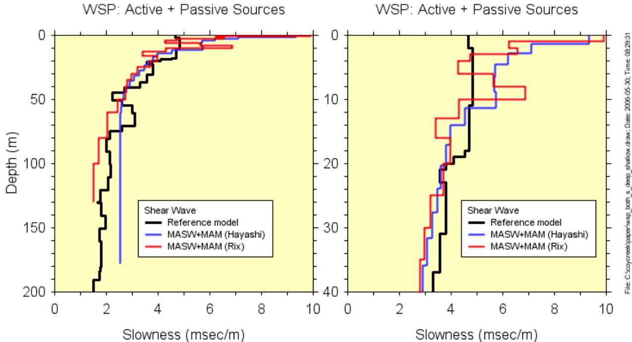
Figure 11. Comparison of reference model and models from combined active--passive source measurements at WSP. An expanded depth scale is used in the right-hand graph to show better the details at shallow depths.
