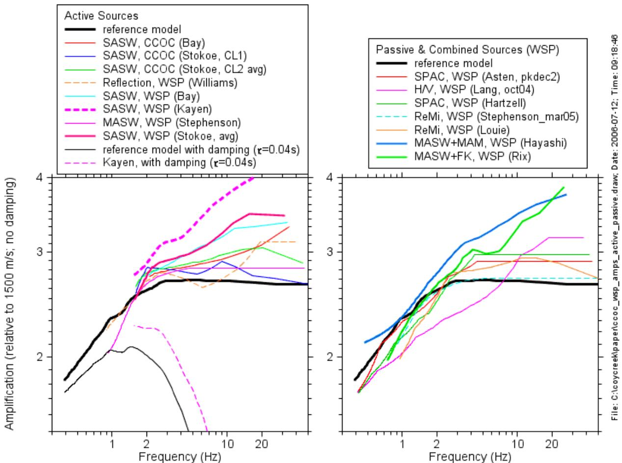
Figure 15. Approximate site amplifications based on square-root-impedance method. The effect of including damping (represented by a factor  $\exp(-\pi\kappa f)$ , where  $\kappa = 0.04s$ ), is shown for two of the models. If it is assumed that the damping for all models is given by this factor, it should be noted that the ratios of amplifications for different models with and without damping is the same.
