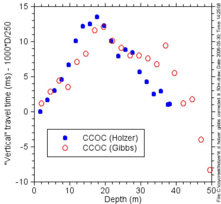
Figure 7. Reduced travel times (corrected for horizontal offset of source from borehole) at CCOC.
