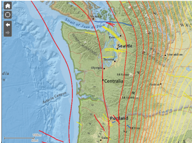
Figure 23. Map showing the location of the two example sites (Seattle and Centralia) used in the PSHA along with the crustal faults (red and yellow lines) and subducting Cascadia subduction zone plate depth contours starting at 20 km depth off the coast and increasing depths of 20 km moving east. Base map and faults from USGS Quaternary Fault GIS webviewer: http://usgs.maps.arcgis.com/apps/webappviewer/index.html
